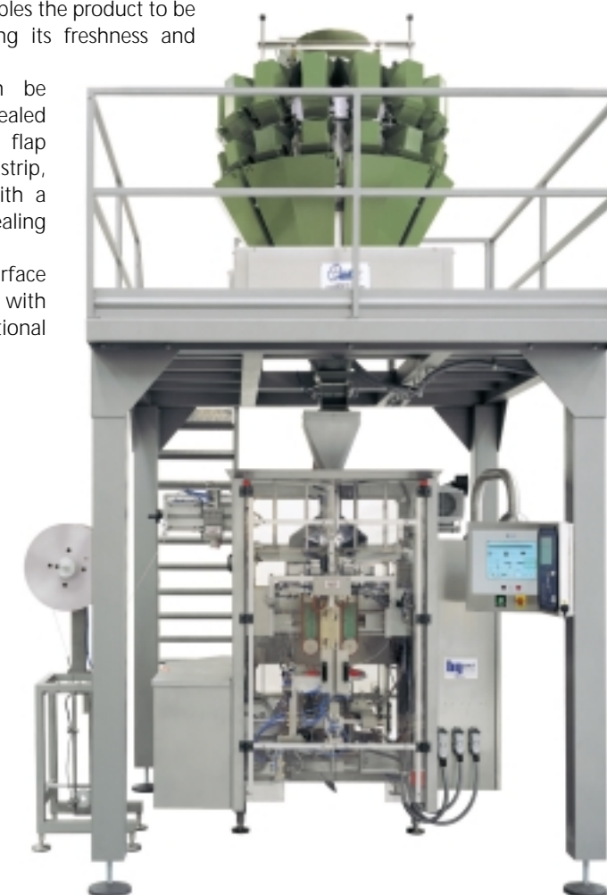
VETTA from BG PACK is a vertical machine, a.o. designed for cheese packaging
