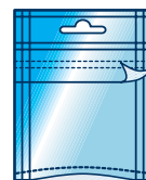
stand-up bag (recloseable) with euro hole punch - from one film - (for dry and heavy products only)
