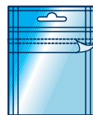
flat bag (recloseable) with euro hole punch - from one film (for dry and heavy products only)
