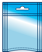
3 side seals stand-up bag with euro hole punch on vertical sealing bar and zip in line
